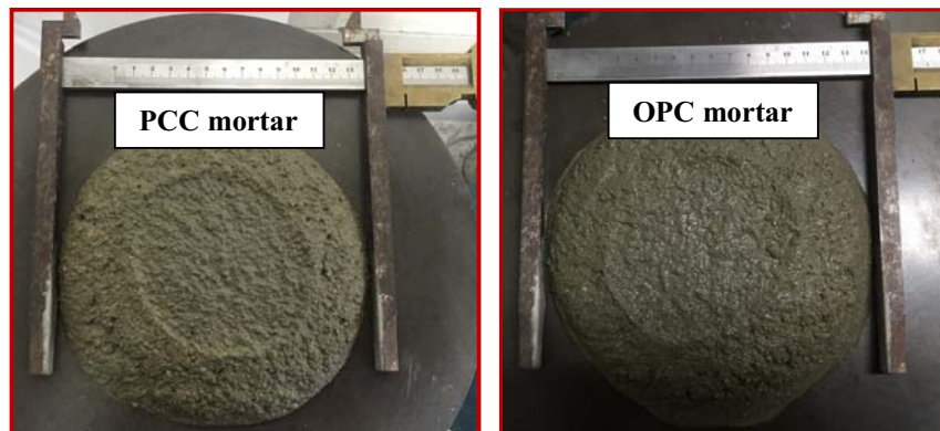
Figure 4. Slump flow of PCC and OPC mortar
